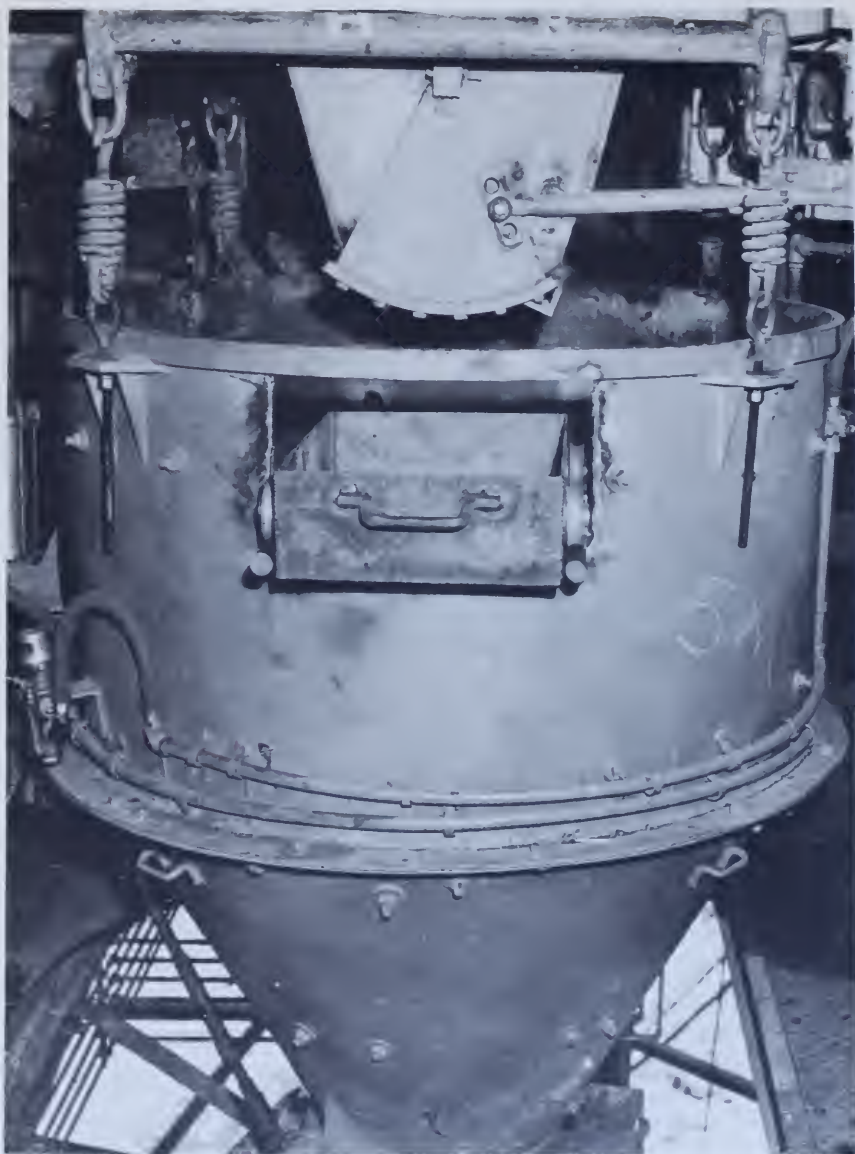
Figure 92.—Aggregate sampling bucket in batcher at mixing plant. Bucket is on rollers for easy removal of sample. PX-D-25253.
